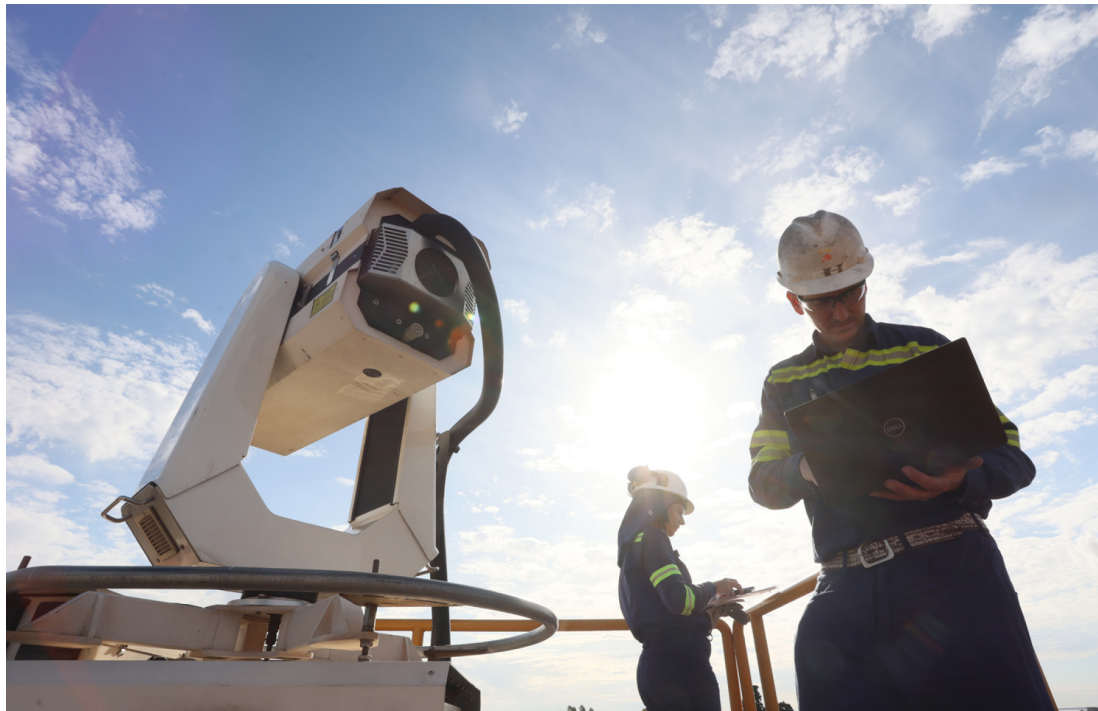
LiDAR (Light Detection and Ranging) technology. Currently undergoing testing at Ternium's San Nicolás unit in Argentina and the Rio de Janeiro unit in Brazil.
